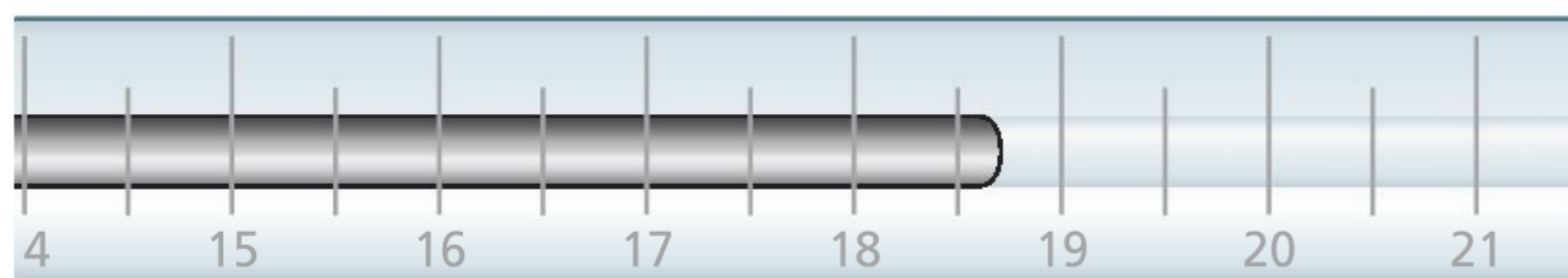
Figure 1.3 A magnified thermometer scale showing a temperature of 18.7°C: the last digit is uncertain
