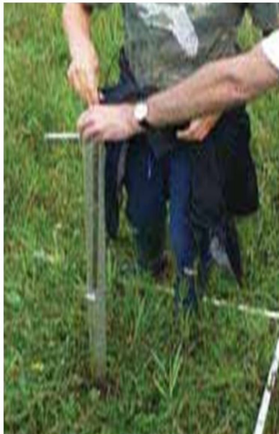
Figure 5.2 Using a simple penetrometer to measure soil compaction. A metal bolt with a pointed end is dropped within a guide sleeve – depth of penetration of soil indicates compaction.
