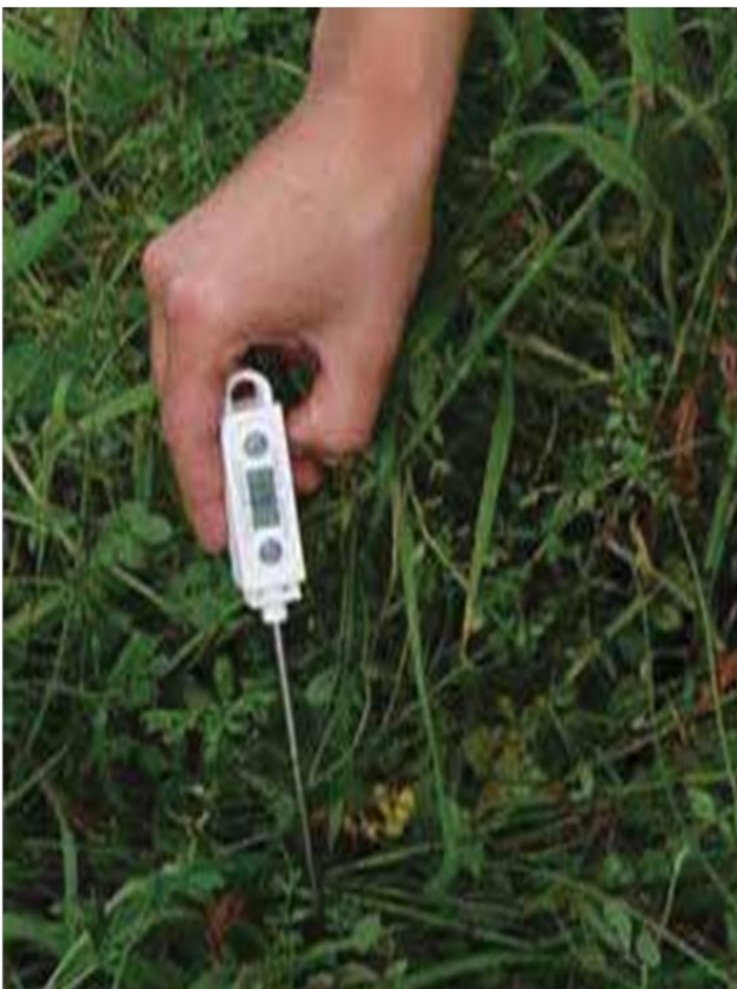
Figure 1.8 A digital thermometer being used to record soil temperature
