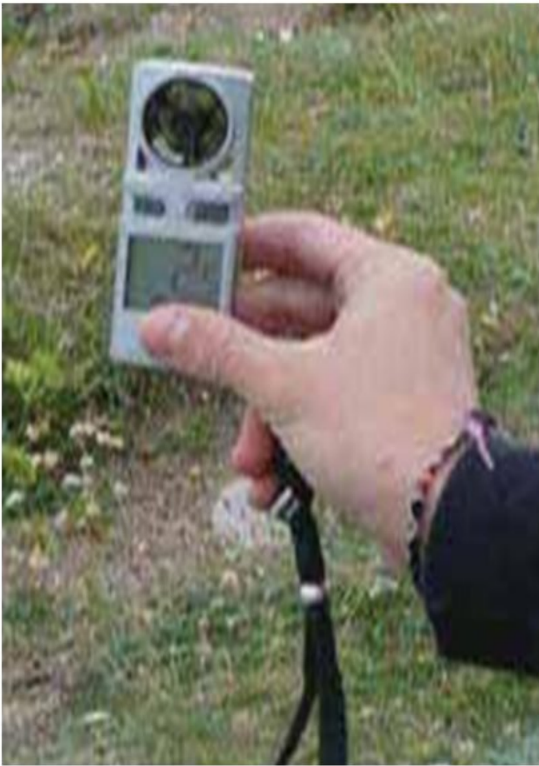
Figure 5.1 Using an anemometer to measure wind speed in a shingle ridge succession
